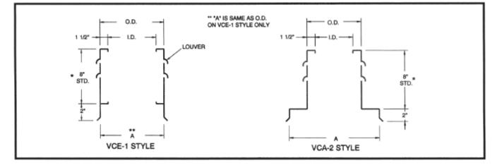
NOTE: WHEN SIZING NECESSARY ROOF CURB FOR ADAPTER, CURB O.D. WILL BE 1-1/2" LESS THAN "A" DIMENSION OF EXTENSION OR ADAPTER. SEE ROOF CURB SECTION FOR PROPER SIZE.
